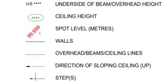
Spot levels are in metres & related to a temporary local datum situated at floor level within the lower basement area (value 100.00m).
